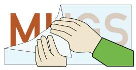
**10.** Remove any air bubbles by puncturing the bubble at one edge with a pin, then squeegee the trapped air towards and out of the puncture.
